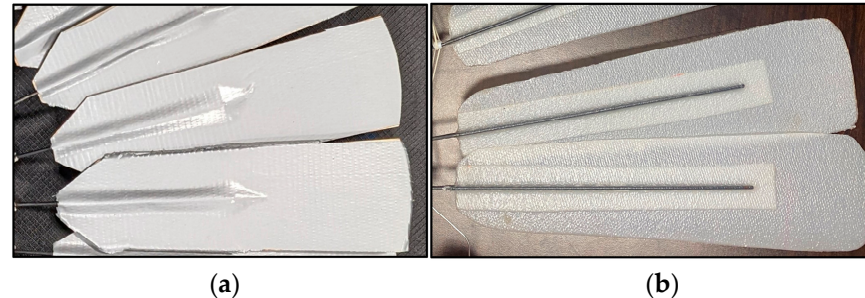
Figure 8. Sample manufactured feathers: (a) reinforced balsa wood, (b) interwoven fiber-glass composite.
